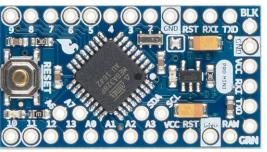
for the FTDI board connection on the right edge. It does not have a power-in jack, but it does include an on-board voltage regulator accessed through the "RAW" connection near the lower right-hand corner of the board
