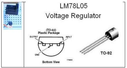
(You should check the voltage with a multimeter before you use one.) The image shows the pinout configuration for a LM78L05 regulator in a standard TO-92 housing. It works perfectly well in place of a step-down converter for this low-power data logging circuit, although its operating current of about 5 mA is a little higher than the current required by the step-down converter. It requires an input voltage of at least 7 VDC and no more than about 35 VDC.
